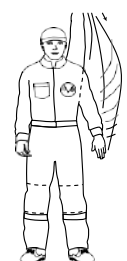
Is it safe to cross the track? Arm vertical: Wait (not safe) Arm lowered: Cross (safe)
