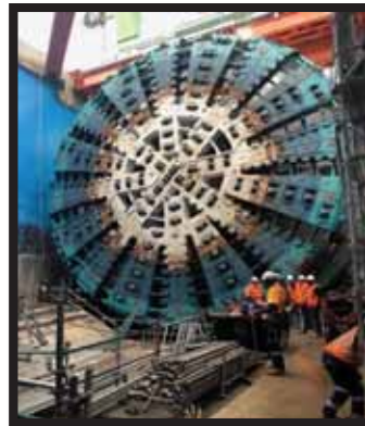
This is the face of the huge Tunnel Boring Machines (TBM) that are currently carving their way under Melb, Sydney & Brisbane as well as the Snowy River Scheme to name but a few.
